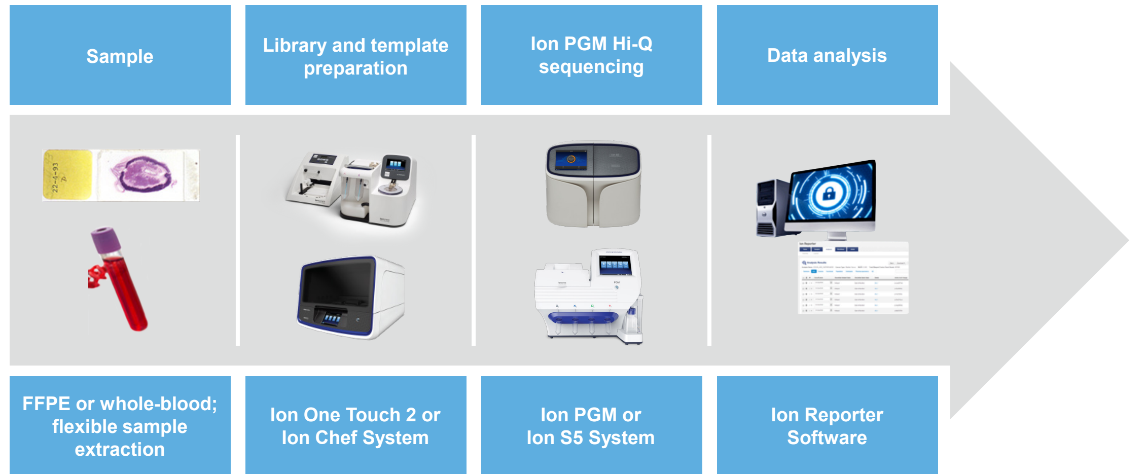
Figure 1. The Ion Torrent™ Oncomine™ BRCA Research Assay workflow leverages the proven performance of Ion AmpliSeq™ chemistry to enable detection of germline and somatic variants from blood and FFPE DNA samples. We demonstrated high sensitivity and specificity for variants at frequency \geq 5\% with only 10–20 ng input DNA.
